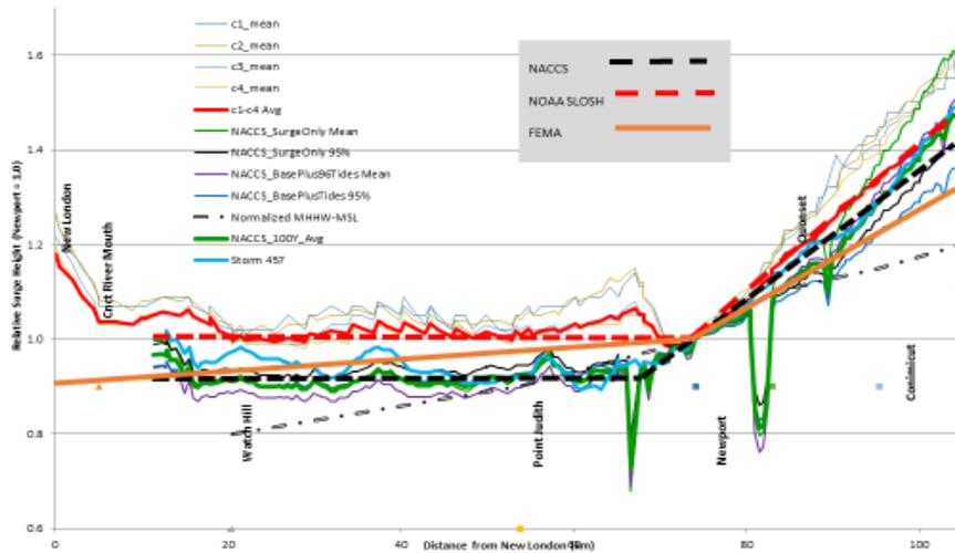
**Figure 5** Peak surge water level vs distance from New London , CT along the southern RI coast line, and up the central axis of Narragansett Bay relative to Newport, RI for NOAA SLOSH and ACOE NACCS simulations. Results are
