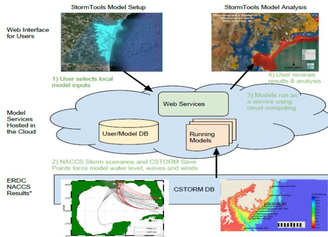
**Figure 1 Vision for STORMTOOL system showing access to NACCS surge model predictions from the CSTORM Data Base.**
