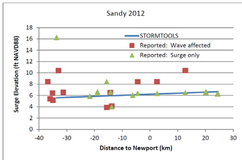
**Figure 2** Peak storm surge water levels (FEMA,2012) for 1938, 1954, and 2012 hurricanes vs distance up the bay referenced to Newport, RI. The data are fitted using a straight line with distance along the central axis of Narragansett Bay. Negative distances are to the west following the southern RI shoreline.
