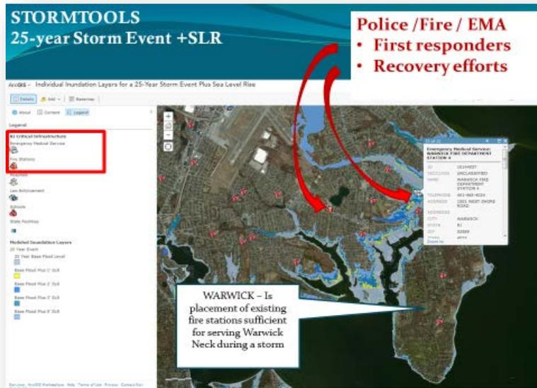
**Figure 7** Flooding map for Warwick Neck, RI showing flooding from the 25 yr return period storm with SLR. The location of critical infrastructure are provided
